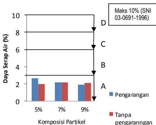
Gambar 1. Histogram daya serap air *paving block*
